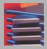
The M100 forms high quality closed corners from a pre-bent flat blank from various Materials such as Mild Steel, Stainless Steel, Aluminum, Brass etc.
