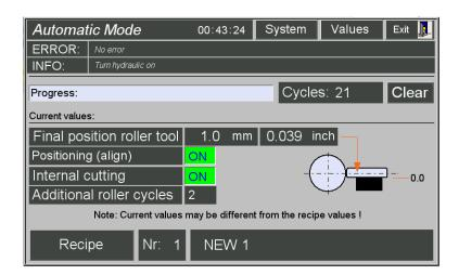
The control surface of the M100 gives you a clear overview of the status of the process and the parameters picked for the forming.
